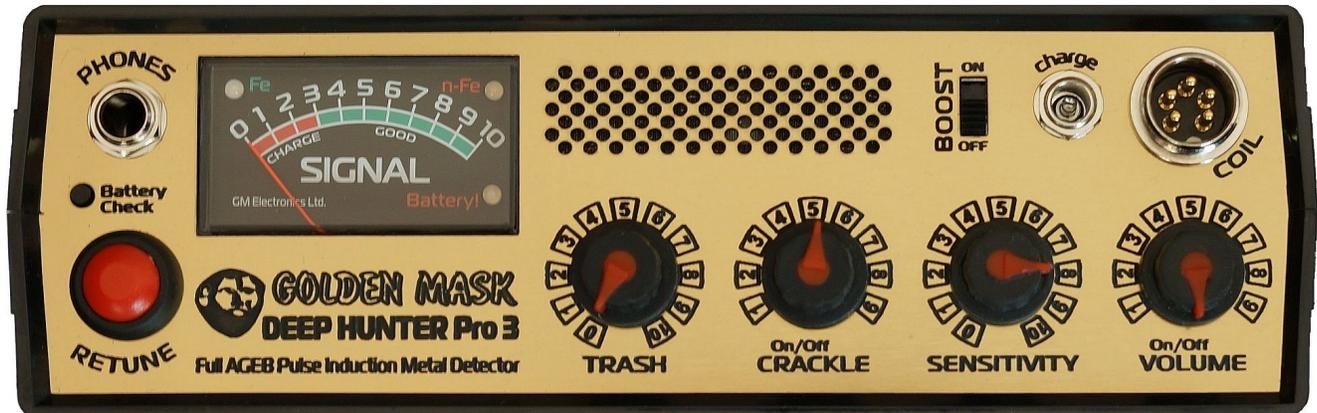
**Golden Mask Deep Hunter Pro3** is a professional metal detector designed to detect deeply buried large metal objects (larger than 8 cm). It has the ability to indicate the type of the metal (ferrous / non-ferrous) and a filter system to significantly reduce interferences caused by power lines.
